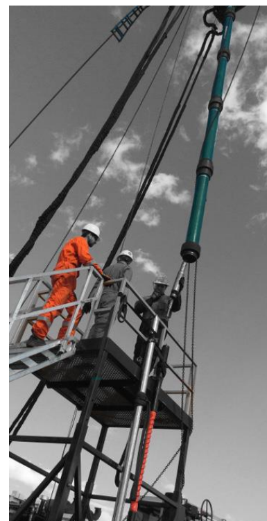
Loading CoilDrive into lubricators
